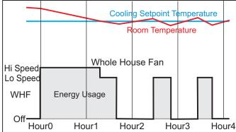
Whole House Fan Operation Using Temperature and Speed Control
