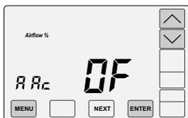
To turn Automatic Airflow Control OFF, touch the DOWN key. The user must set the airflow when airflow control is off.
