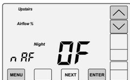
Touch the UP key to turn the option ON. Touch the DOWN key to turn the option OFF.
