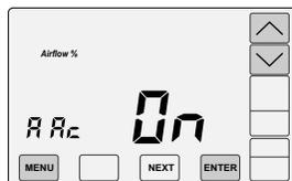
Thermostat defaults to Automatic Airflow Control On and automatically directs more airflow to where it's needed.
